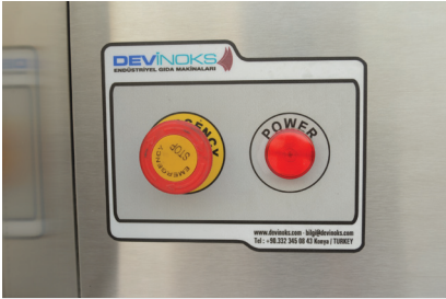
Enerji Göstesgesi ve Acil Stop Indicator Power & Emergency Stop
